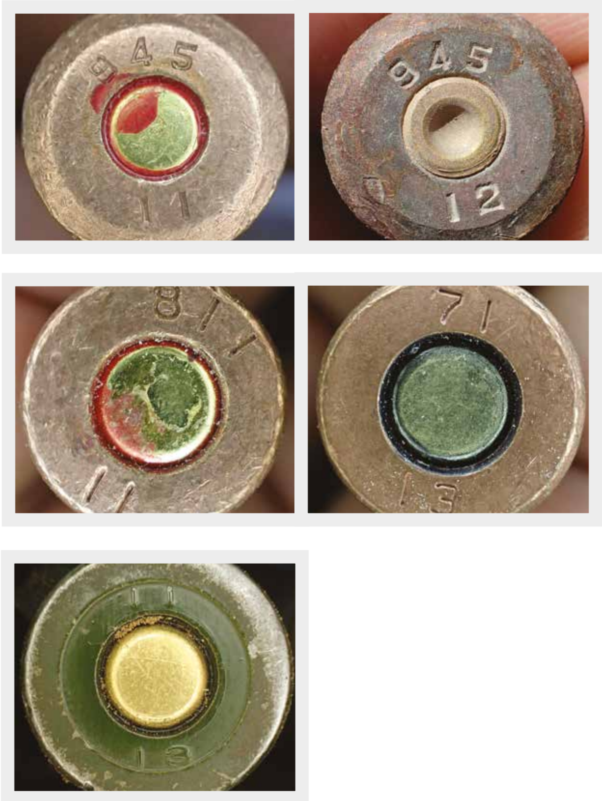
Figure 10 Embargo-year and post-embargo Chinese-manufactured ammunition documented in Sebha, Libya, July 2015: 7.62 x 54R mm (top row), 7.62 x 39 mm (middle row), and 12.7 x 108 mm (bottom)
